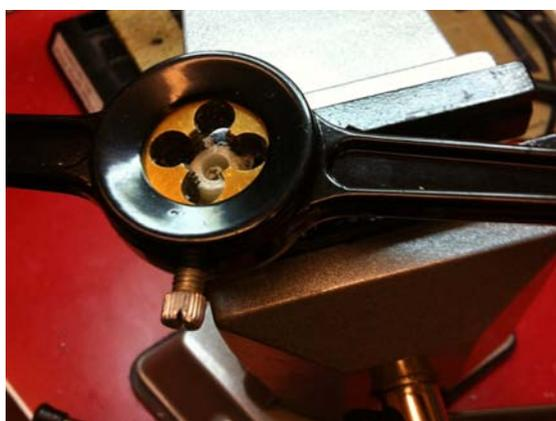
Figure 9: Threading one of the Spine's collars.
