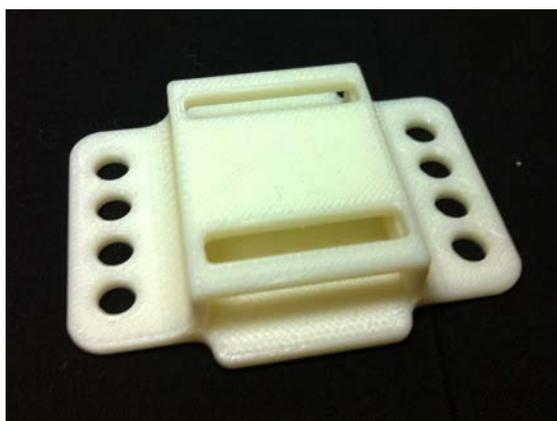
Figure 5: One of the Rib mounts. The holes on the side of the mount are for sewing the mount onto the dancers' corsets.
