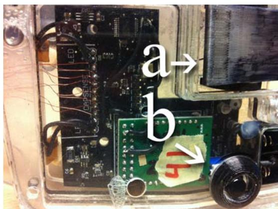
Figure 11: The electronics enclosure of a Rib, showing the location of a) the clip and b) the dome surrounding the power button. The clip was colored via Sharpie, the dome with spray paint.
