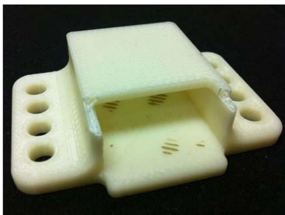
Figure 6: A mount where the top has come unsecured from the sides.
