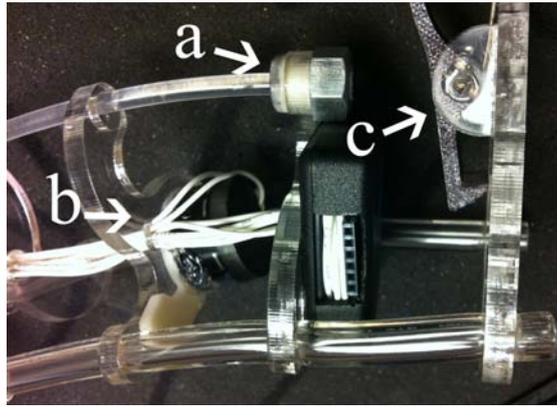
Figure 10: The top of the spine, showing the locations of: a) the PET-G collar, b) the lighting with its printed mounting collar and top, and c) the clip.
