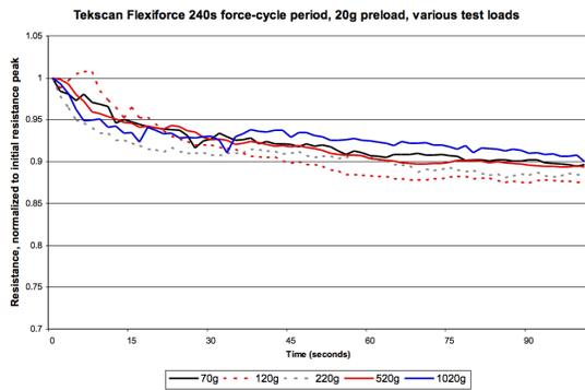
Figure 2: Dead weight drift for the three samples, period of 240s.
