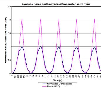
Figure 5: Variation of conductance (normalized) with applied force for the FSR and PS3.
