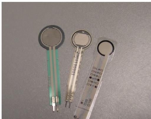
Figure 1: Three touch sensors from Interlink, LuSense and Tekscan.
