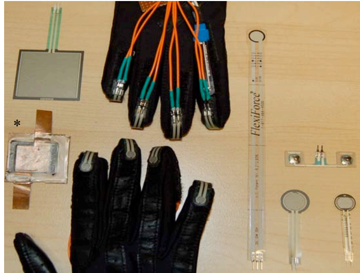
Figure1: Various pressure sensors to be used or mounted onto a glove for musical application. One can also notice an example of homemade paper FSR on the left*.
