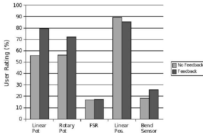
**Fig. 2.** User ratings for each sensor both with and without visual additional feedback
