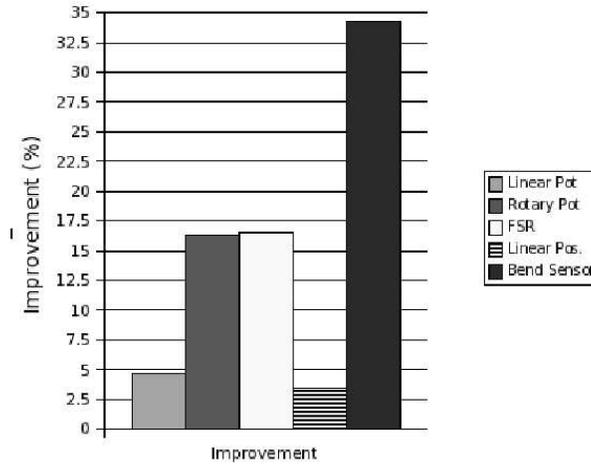
**Fig. 4.** Improvement in user accuracy for each sensor, relative to their initial accuracy
