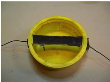
Figure 3 Multi-Couch Bend sensor: a pigment line is stuck between two latex layers making a sort of tube
