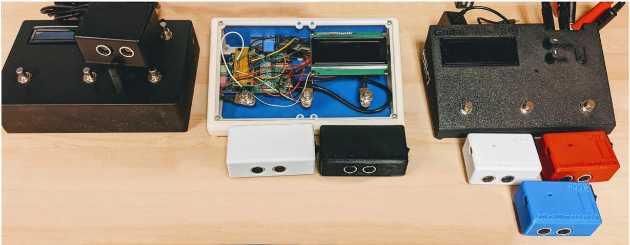
**Figure 3.3** Current GuitarAMI versions and their modules: version 4 (left), version 5 (center), and version 5a (right). Version 4 is based on Prynth and runs SuperCollider code, while versions 5 and 5a use a modified Linux distribution capable of running SuperCollider code, Pure Data patches, audio plugins in LV2 format, and custom software installed by the user.
