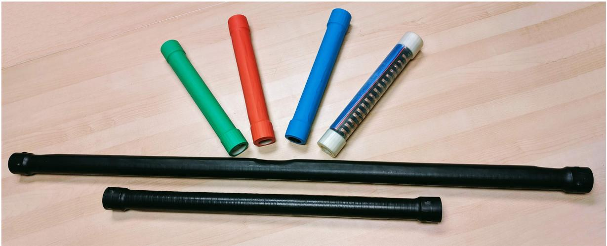
**Figure 3.1** T-Stick instrument “family” including wireless 2nd generation (2GW) Sopraninos (30 cm in length) on top, wired 2nd generation (2G) Tenor (120 cm in length) in the middle, and wired 2nd generation (2G) Soprano (60 cm in length) on the bottom (Meneses, Fukuda, and Wanderley 2020).
