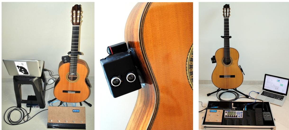
(a) First GuitarAMI prototype used in live performances, built using a wired sensor module, DSP unit, audio interface, and laptop. (b) Wireless RF GuitarAMI sensor module using an Arduino Nano. This module replaced the wired module between versions 2 and 3. (c) Third GuitarAMI prototype, redesigned to have a modular system and simultaneously improve portability and setup time.
