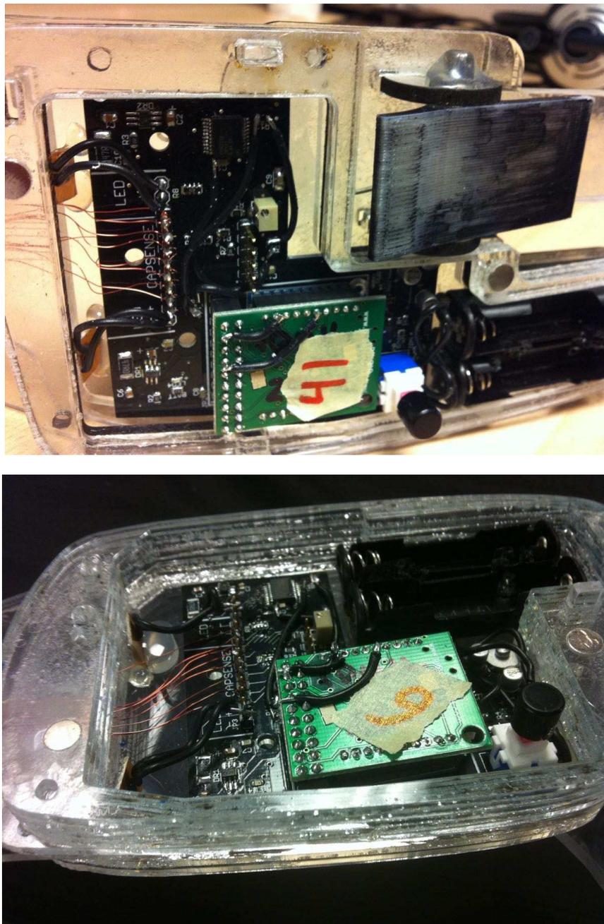
**Fig. 3.7** The PCB and acrylic enclosure were designed at the same time in order to ensure a perfect fit. While most of the electronics were incorporated on the PCB, the LEDs and battery holders were mounted separately in order to allow for flexible position. (top) the electronics enclosure in the Rib, with the LEDs on the left positioned to shine down the length of the Rib. (bottom) the electronics enclosure in the Visor, showing the different location for the battery holder.
