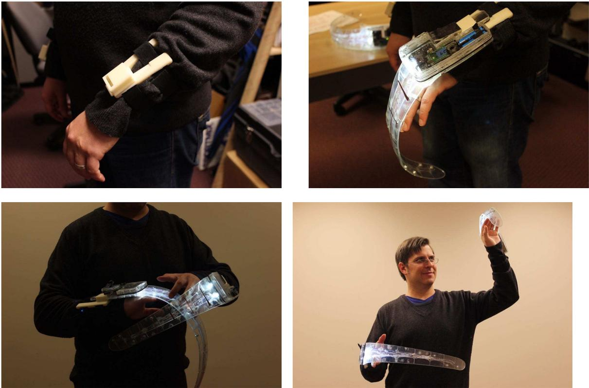
**Fig. 3.15** The mounts used in the quadcopter project. Clockwise from top left: a) A mount attached to an arm. b) A mount with a Rib inserted. c) Playing the Rib using the capacitive touchpads. d) Playing the Rib using motion data.
