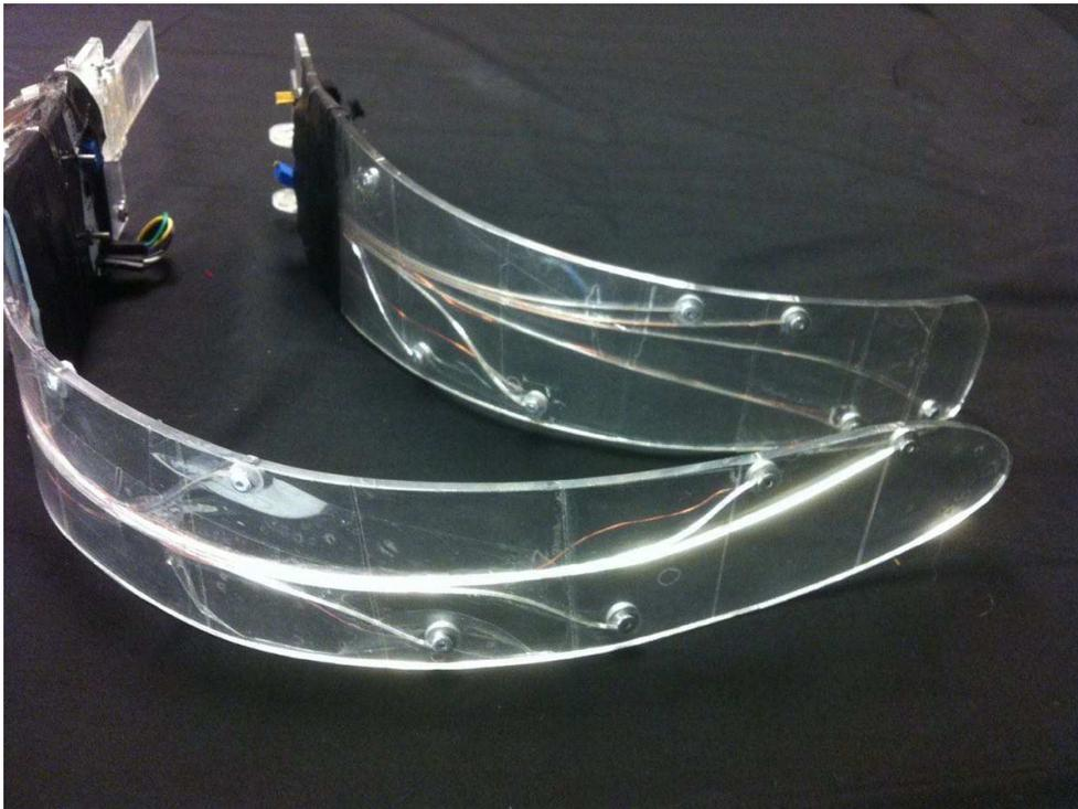
**Fig. 3.18** The first two Ribs created using magnet wire. Notice the black gaffers tape attempting to compensate for cracks in the acrylic.
