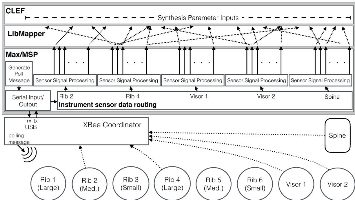
**Fig. 3.9** The signal flow for the Prosthetic Instruments as used in *Les Gestes*. Blocks within the grey border are software environments located within PCs.
