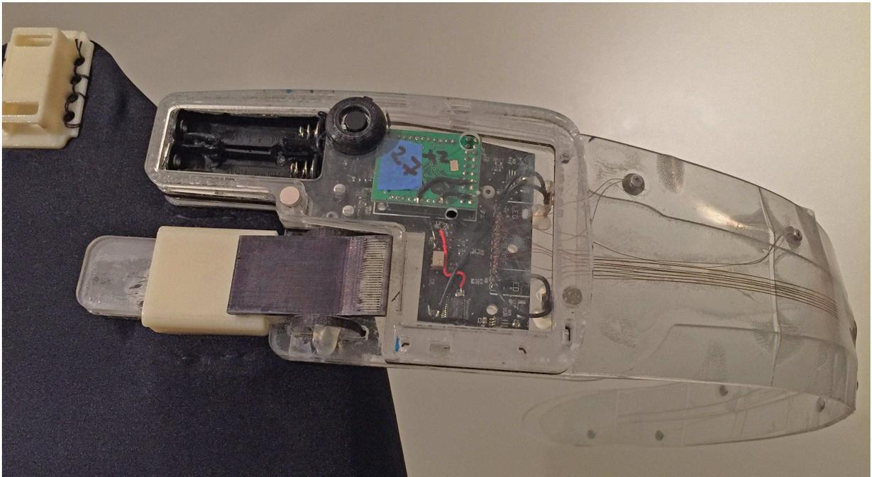
**Fig. 3.10** The mounting system designed for the Prosthetic Instruments. On the top left is a 1/2" mount, with the holes provided for sewing to the garment and the slot for the clip easily visible. The mount for the Rib has fabric covering the sew holes.
