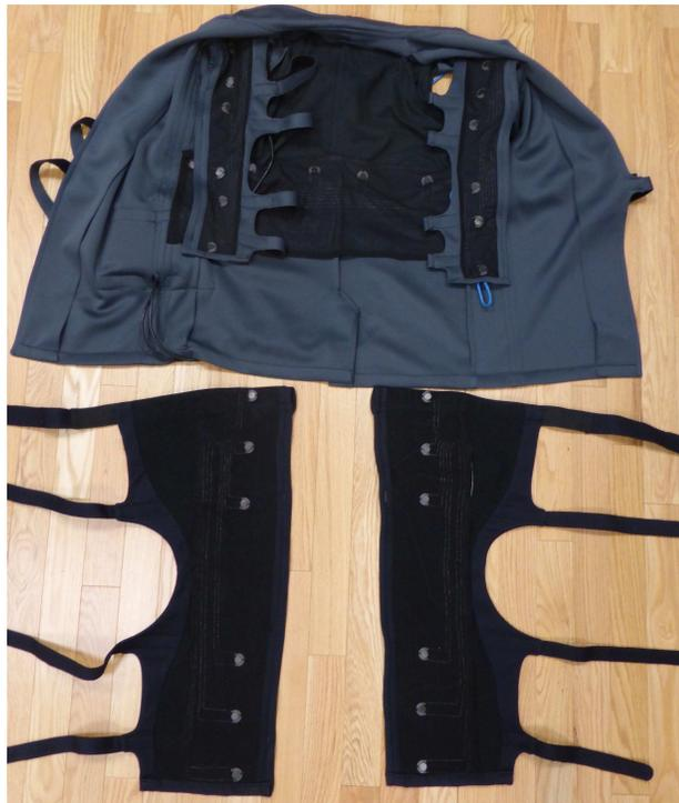
**Fig. 4.1** A view of the *Ilinx* garment from the inside. The actuators are visible as silver circles running down the length of each limb and horizontally on the torso. The open design of the arms and leggings are also visible.
