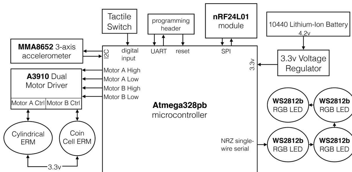
**Fig. 5.2** A system overview showing the hardware configuration of a single VibroPixel.
