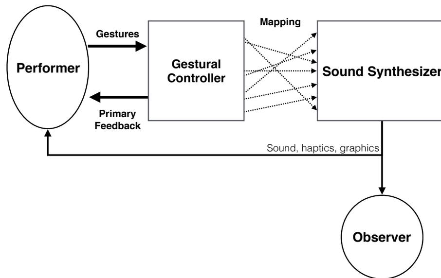
**Fig. 2.1** A simplified model of typical DMI design, based on Bongers (2000, 45), Miranda and Wanderley (2006, 3), and Marshall (2008, 23).
