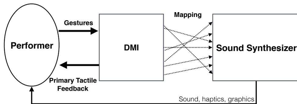
**Fig. 1.1** A simplified model of a digital musical instrument, based on Bongers (2000, 45).
