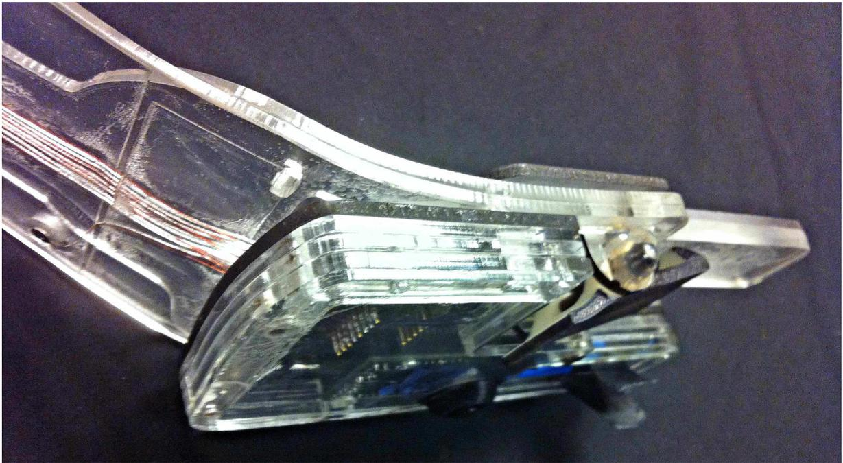
**Fig. 3.6** Detail showing the laminate construction of the Ribs, with the protrusion and clip for mounting visible on the right. The polycarbonate layers are easily identified by their brown edges.
