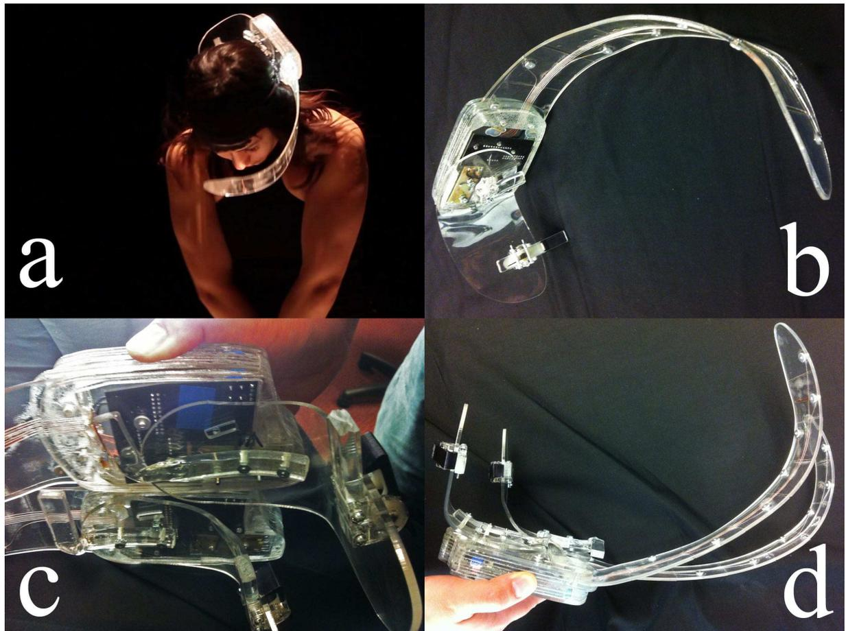
**Fig. 3.2** Clockwise from top left: Soula Tragoukos wearing the Visor; a view of the Visor in which the mounting panel is clearly visible; the different shapes of the Visors formed for each dancer; and a closer look at the different shapes of the Visors' and their mounting panels.
