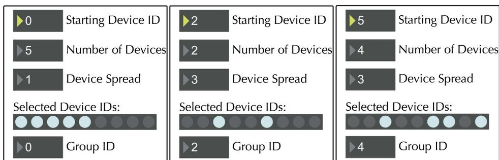
**Fig. 5.7** An interface for algorithmic generation of Device IDs. Three examples are presented with different settings for starting Device ID, Number of Devices, and Device Spread. Below the controls for setting these parameters is a visual representation of the currently selected devices. Also shown is the currently selected Group ID.
