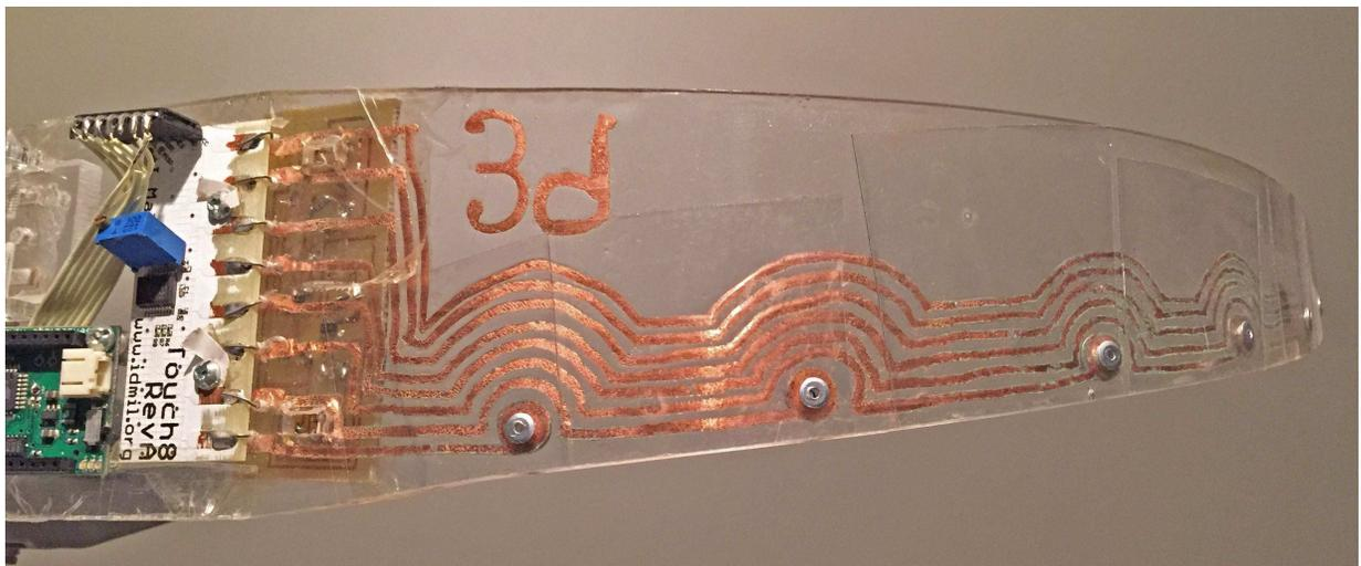
Fig. 3.17 A Rib prototype created with etched copper traces and transparent conductive plastic touchpads.
