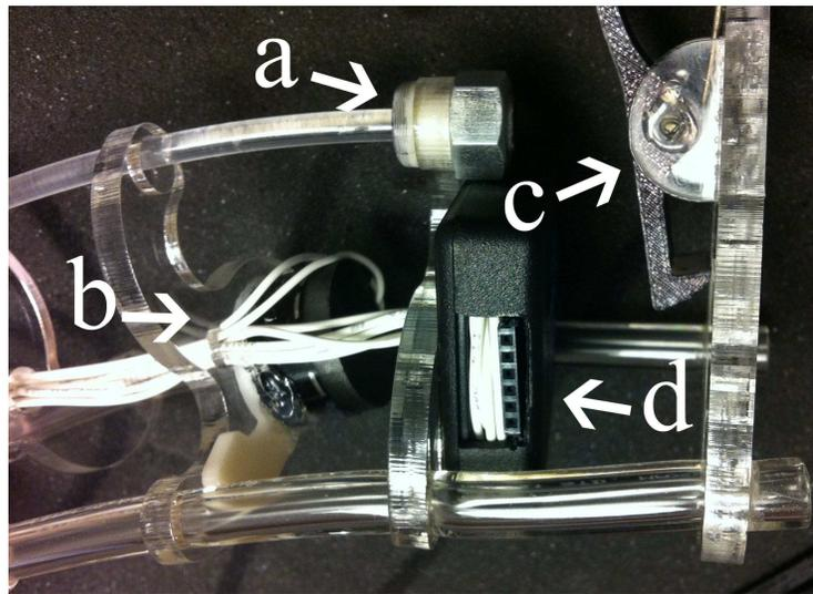
**Fig. 3.8** The top of the Spine, showing various features: a) the Pet-G rod secured to the second-to-the-top vertebrae using a 3D-printed mount; b) the wiring for the sensor board coming through the central hole of a vertebrae; c) the mounting clip; and d) the sensor board in its plastic enclosure.
