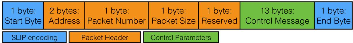
Fig. 5.4 Overview of a complete VibroPixel wireless packet.
