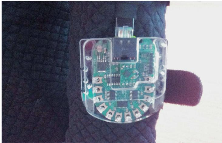
**Fig. 4.3** The driver boards on the *Ilinx* garment incorporate circular terminals for embroidering conductive thread which connects to the actuators. At the top of the board is an RJ45 jack for the Cat5 cable which connects to the central control unit. Protecting the driver board is a laser-cut, solvent welded clear acrylic enclosure.
