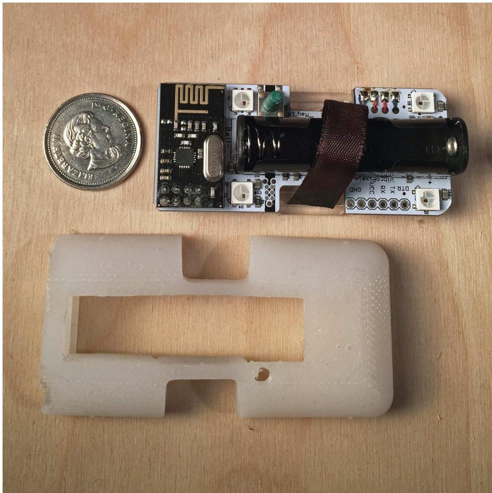
**Fig. 5.1** A top view of a VibroPixel and its silicone cover.
