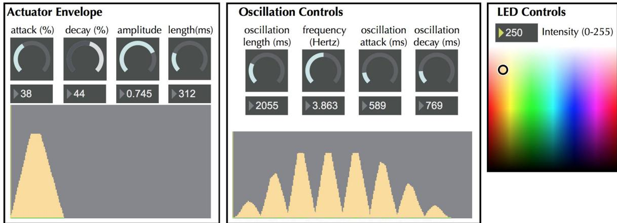
**Fig. 5.6** An example user interface for generating control parameters for the VibroPixels, with sections for setting parameters for the actuator envelope, oscillation function, and LED functionality. The UI includes a visual representation of the results of the current settings both for the actuator envelope and the oscillations.
