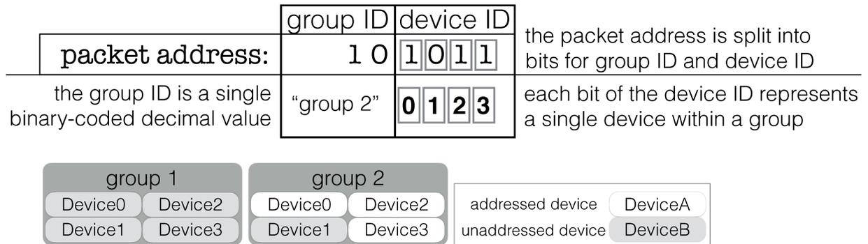
**Fig. 5.3** Example of the VibroPixel addressing scheme using a 2-bit group ID and 4-bit device ID. In this example, the packet is addressed to devices 0, 2, and 3 in group 2.
