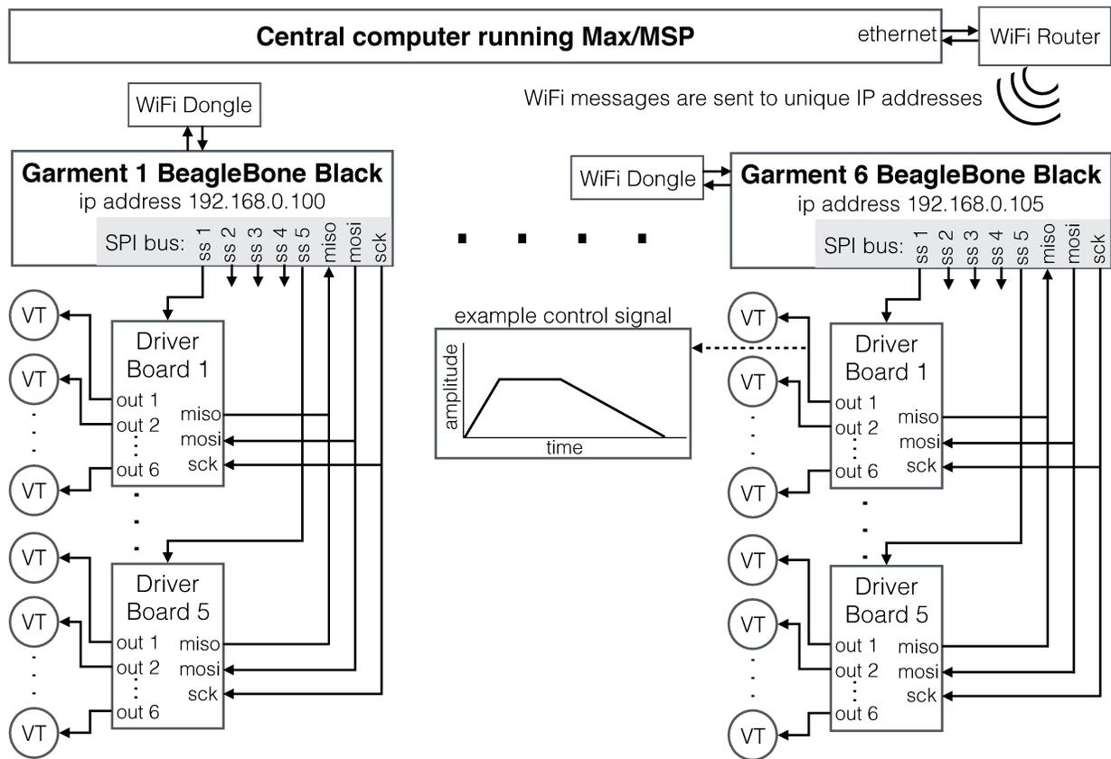
**Fig. 4.5** A diagram of the network configuration for the *Ilinx* garment. Six garments were used in *Ilinx*, each consisting of five sections, each section with its own driver board and actuators. An example control signal is also shown, illustrating the attack-sustain-decay envelopes used for control of the actuators.
