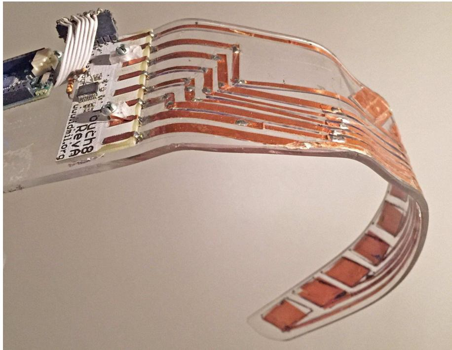
Fig. 3.16 One of the first functional Rib prototypes, with copper touchpads and traces.
