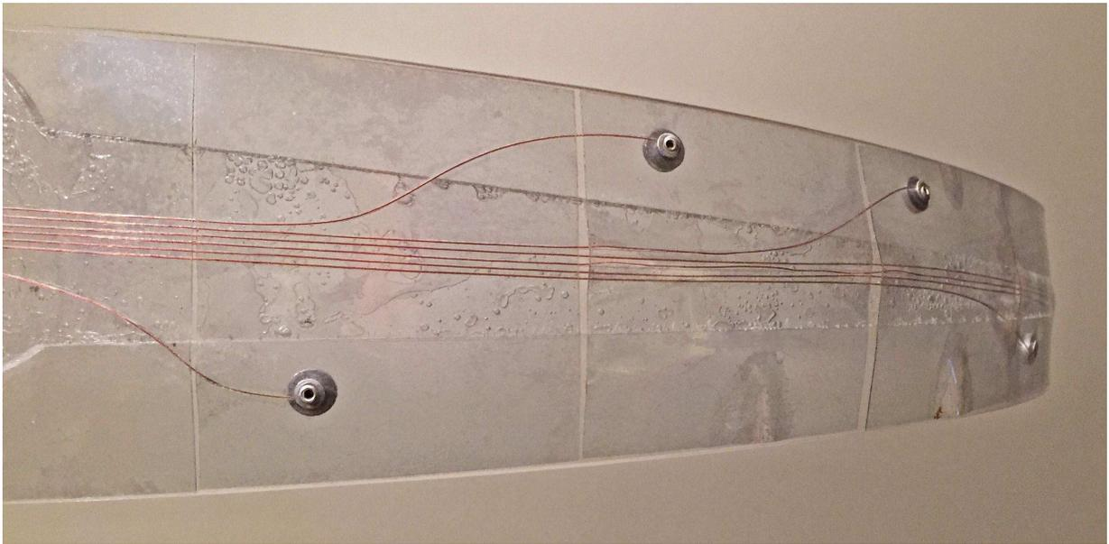
**Fig. 3.4** A closeup of a Rib, showing four touch panels, the magnet wires, and rivets.
