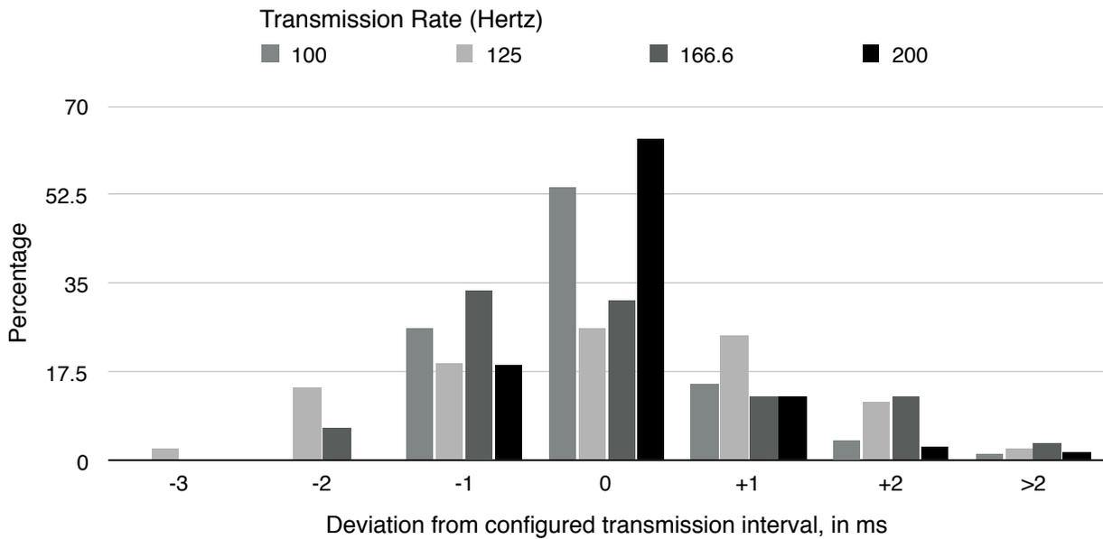
Fig. 5.11 Transmission rate jitter at various rates. The percentage of packets received for each interval between packets is shown for transmission rates between 100 and 200 Hertz.
