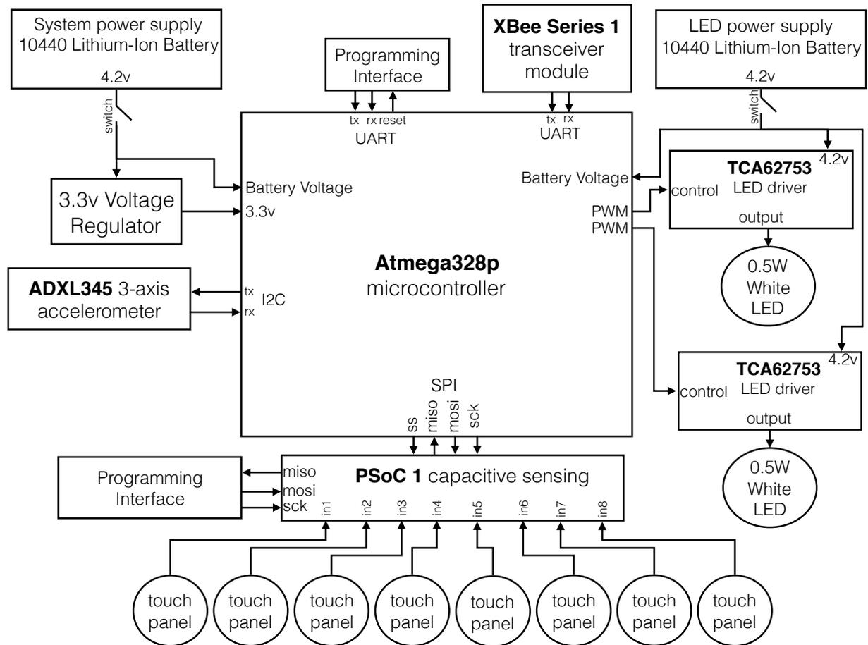
**Fig. 3.3** A block diagram of the electronics for the Rib and Visor.
