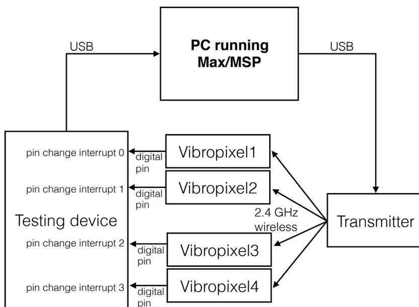
**Fig. 5.12** The configuration of test 3, showing the connection of VibroPixels to the testing device.
