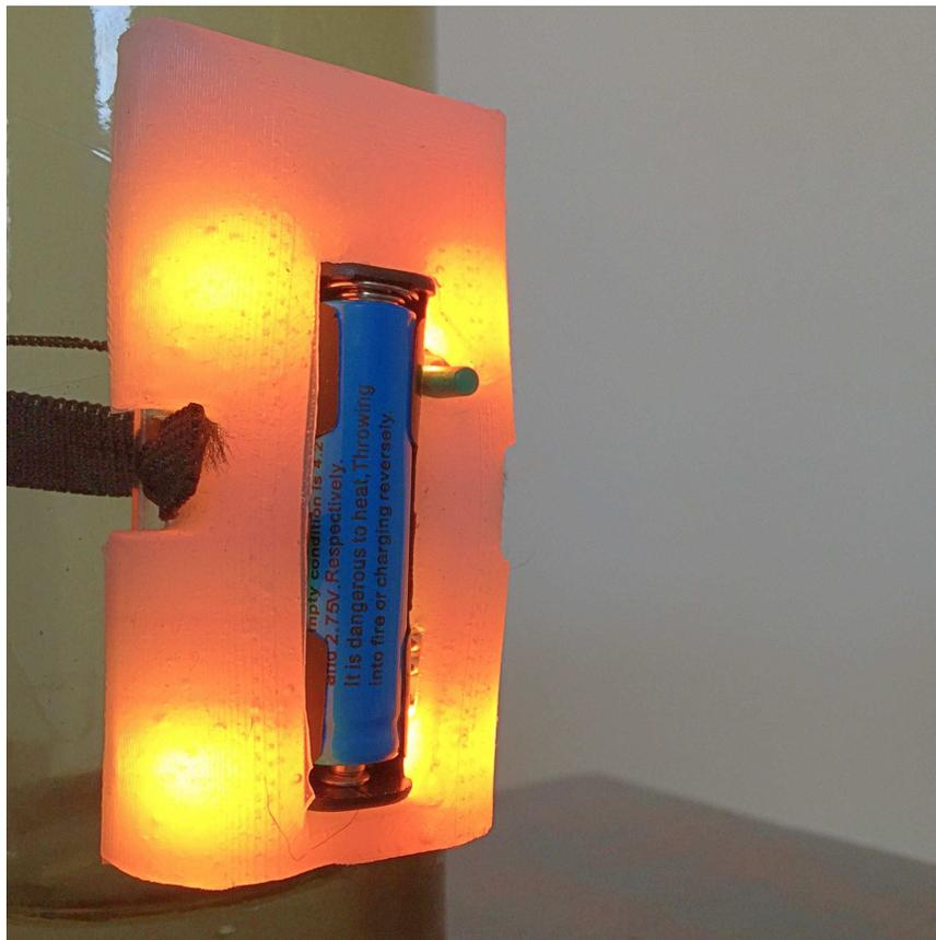
Fig. 5.15 The silicone cover of the VibroPixel diffusing the LEDs.
