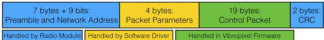
Fig. 5.5 Detail of the VibroPixel control packet structure.
