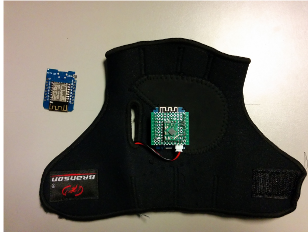
Figure 5.2 Glove with motion sensor and Wemos D1 microcontroller board to capture cellist bowing gestures (Node 1)
