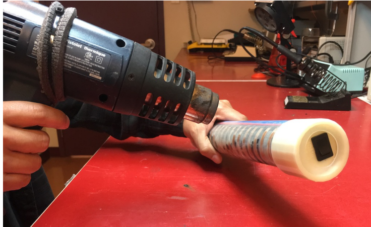
Figure 4.4 Finishing the construction of the Sopranino 2GW-181 by wrapping it with transparent heat-shrink tube.
