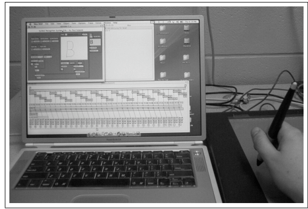
Figure 2: HMM symbol patch with a Wacom tablet input—recognition process.
