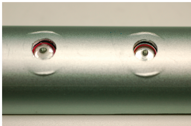
Figure 3. Two toneholes with vibrotactile actuators. The small metal dot in the center of each actuator is a load which lowers the diaphragm’s resonant frequency and increases inertia [30].
