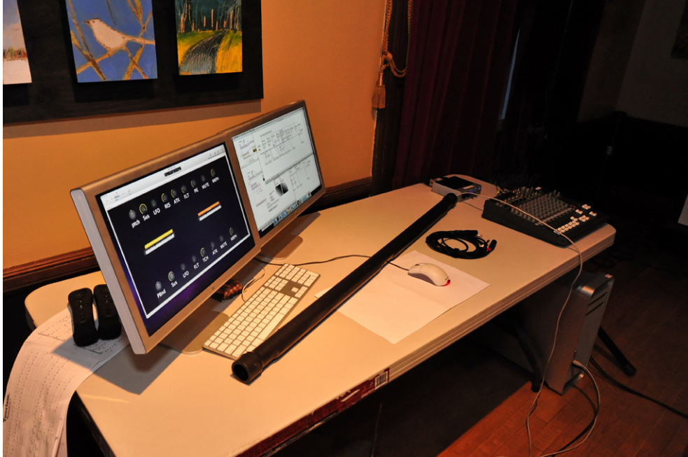
Fig. 2.1 Soprano T-Stick picture from Joseph Malloch’s Blog. It shows T-Stick and the MaxMSP patch, which performs gesture acquisition, mapping, and sound synthesis. URL: https://josephmalloch.wordpress.com/portfolio/tstick . Accessed 18 Oct. 2021
