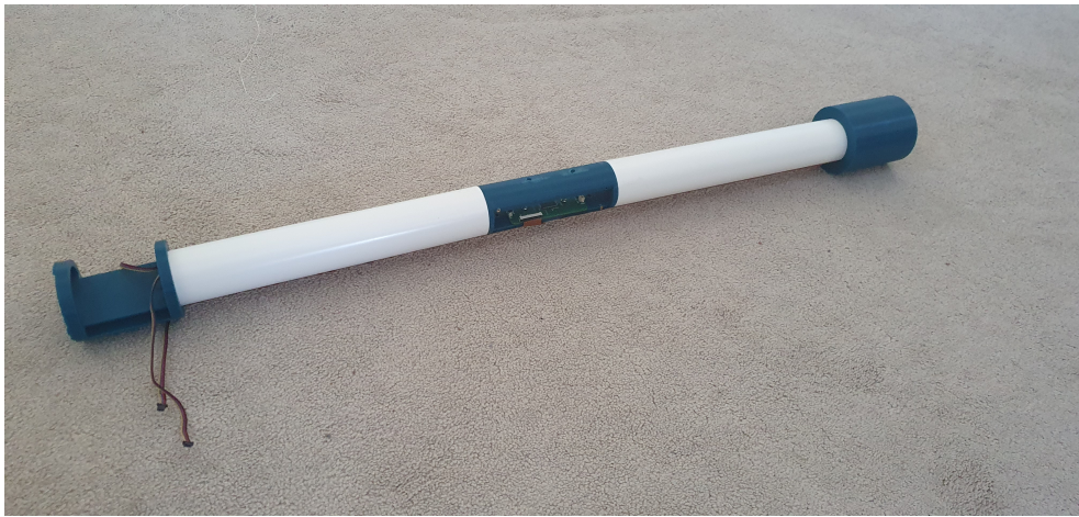
Fig. 5.9 Partially assembled Soprano T-Stick 5GW, the touch board bed and endcap are glued onto the plastic pipe.
